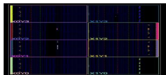
Fig. 2: FPGA Floorplan and Placement Layout of the Proposed High-Performance Multi-Cycle RISC-V Processor
