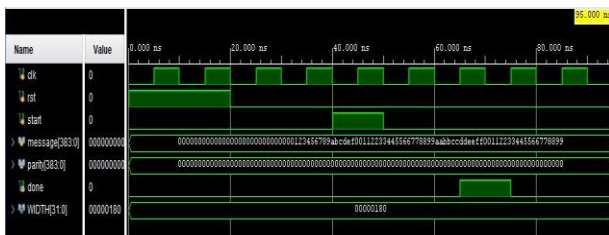
Fig. 4 :Behavioral Simulation Waveform of the Proposed Single-Cycle QC-LDPC Encoder
