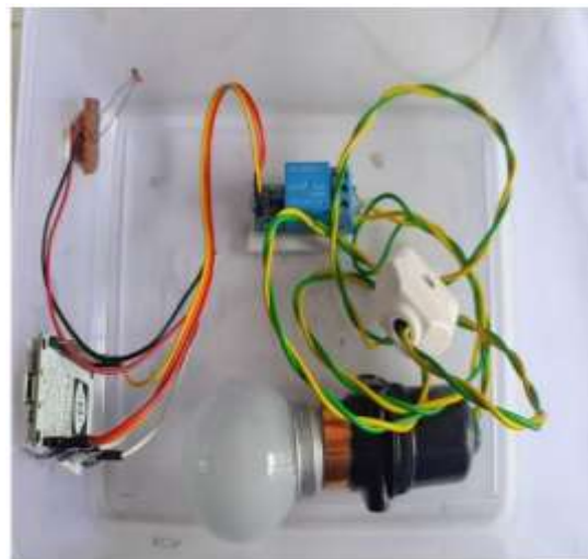
Figure 7: Prototype of the IoT based smart street light system
