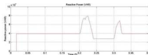
Fig. 15: Grid reactive power under faulted condition
